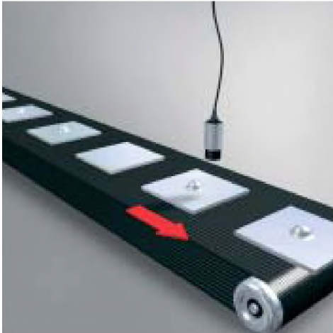
Height and step detection
